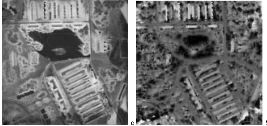
Fig. 4. Confidences ( a ) for the reconstructed DEM to get the refined DEM ( b )
