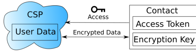
Fig. 6. A contact can access or modify data at a user’s CSP. Therefore, the contact needs an access token and an encryption key.
