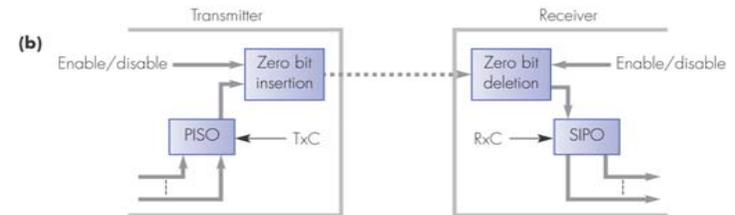
**Figure 1.22** Bit-oriented synchronous transmission: (b) zero bit insertion circuit location
