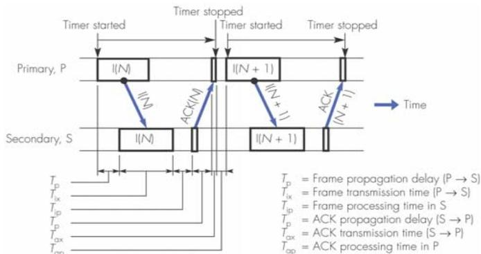
Figure 1.24 Idle RQ link utilization
