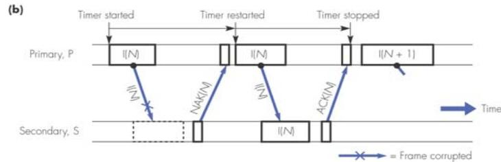
Figure 1.23 ARQ error control scheme: (b) corrupted I-frame
