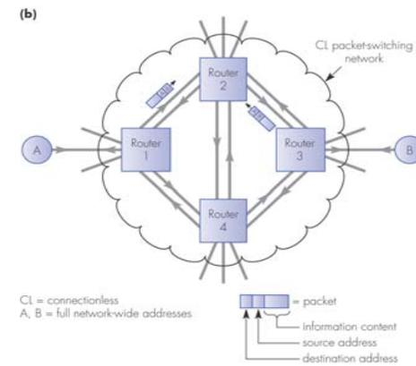
Figure 1.6 Packet-switching network principles: (b) connectionless
