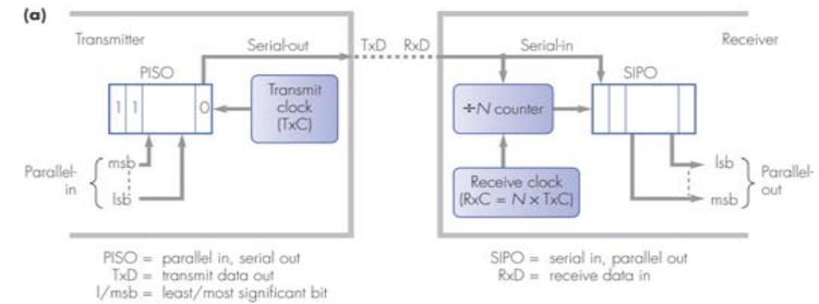
**Figure 1.15** Asynchronous transmission: (a) principle of operation
