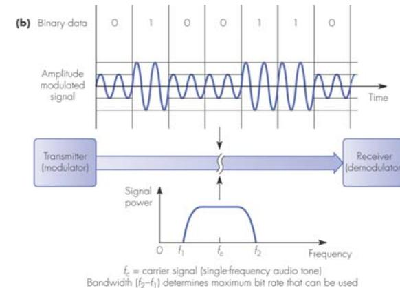
Figure 1.8 Modes of transmission: (b) modulated transmission
