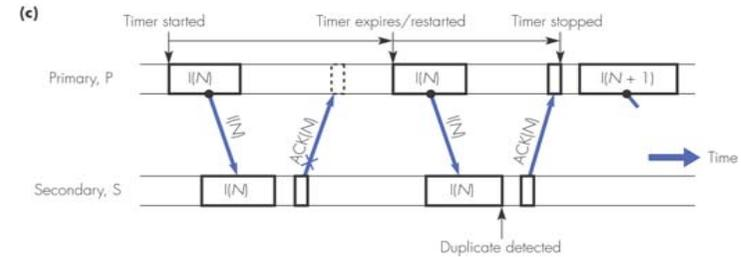
Figure 1.23 ARQ error control scheme: (c) corrupted ACK-frame
