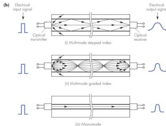
Figure 1.11 Optical fiber transmission media: (b) transmission modes
