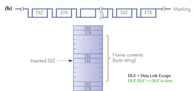
Figure 1.17 Frame synchronization with different frame contents: (b) string of bytes
