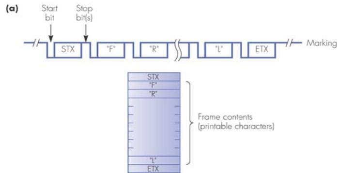
Figure 1.17 Frame synchronization with different frame contents: (a) printable characters
