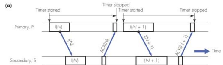
**Figure 1.23** ARQ error control scheme: (a) error free
