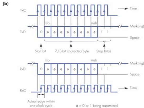
**Figure 1.15** Asynchronous transmission: (b) timing principles
