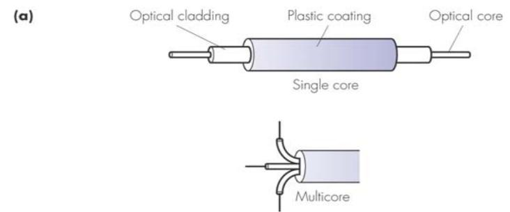
Figure 1.11 Optical fiber transmission media: (a) cable structures
