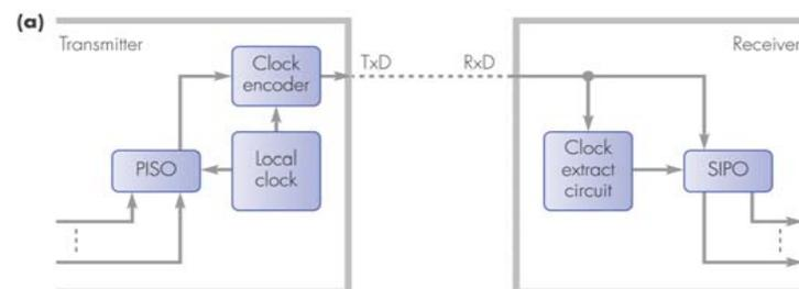
Figure 1.18 Alternative bit/clock synchronization methods with synchronous transmission: (a) clock encoding
