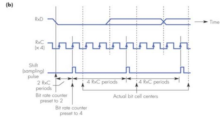
**Figure 1.16** Examples of three different receiver clock rate ratios: (b) × 4
