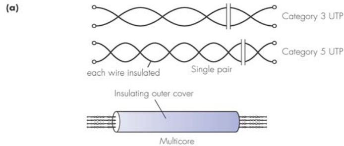
Figure 1.10 Copper wire transmission media: (a) unshielded twisted pair (UTP)
