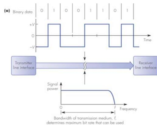
Figure 1.8 Modes of transmission: (a) baseband transmission
