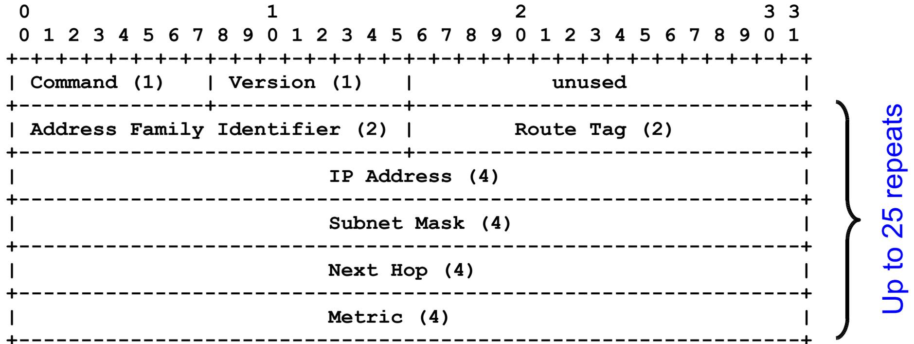
Get used to this form of protocol data unit drawing – it's how all basic Internet standards show bits and bytes. This shows 24 bytes in 6 rows of 4 bytes.
