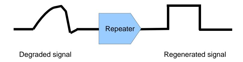
An Ethernet repeater works in both directions
