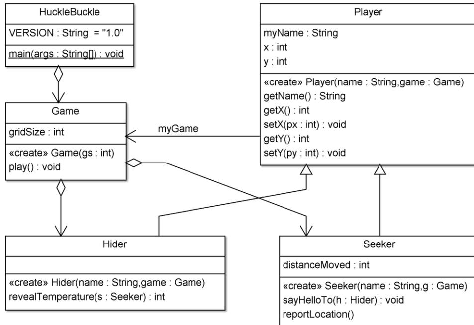
Figure 1. Class diagram for `hbbv1`.
