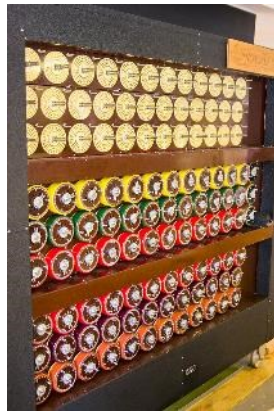
Rotating drums on the Bombe
